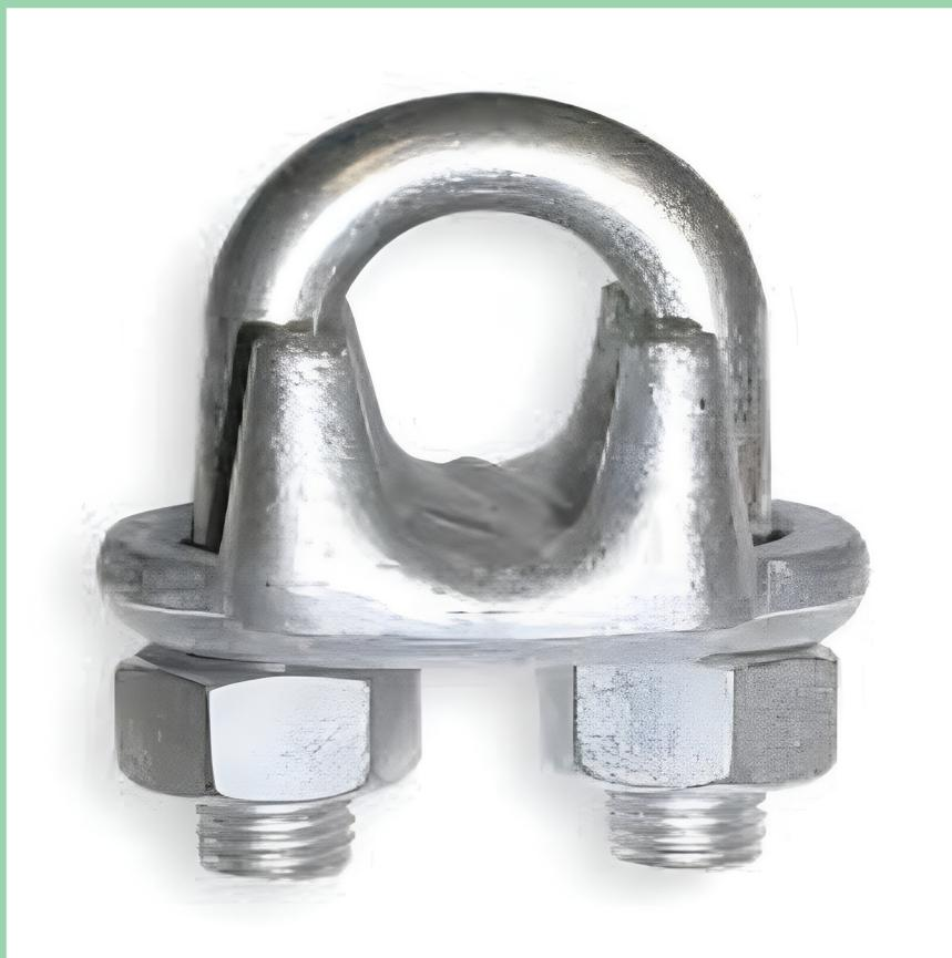
WIRE ROPE CLAMPS THAT ARE USED TO FIX THE LOOSE END OF THE LOOP BACK TO THE WIRE ROPE. IT CONSISTS OF A U-SHAPED BOLT, A FORGED SADDLE AND TWO NUTS. THREE OR MORE CLAMPS ARE USUALLY USED TO TERMINATE A WIRE ROPE. AVAILABLE IN STANDARD SPECIFICATION, THESE CAN ALSO BE CUSTOMIZED AS PER THE REQUIREMENTS OF OUR CLIENTS. THESE FIND APPLICATION IN VARIOUS INDUSTRIES SUCH AS CONSTRUCTION INDUSTRY, CEMENT PLANT, CHEMICAL INDUSTRY AND OIL INDUSTRIES.
